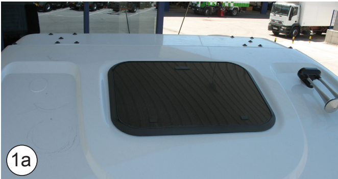
Stralis Cabin before 2008: 40 x 40 EPDM joint
