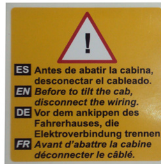
Attach in a visible place at the back of the cabin, next to the top and bottom cable connection
