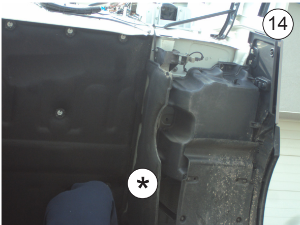
Dismantle guard (*) and move wiring under the protector.
